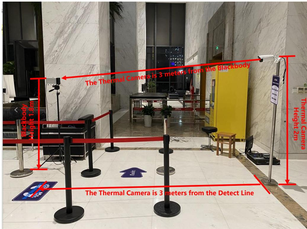
**Note:** the environment is a temporary test point, and the gate is closed. During field installation, direct connection with the outdoor shall be avoided, otherwise the temperature measurement may be inaccurate at the best temperature measurement point due to the influence of indoor and outdoor airflow convection
