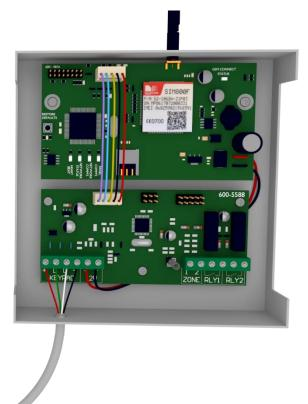
The serial connection between the SMS Duo V2 module and the 805 Alarm Panel is shown in the image above.
