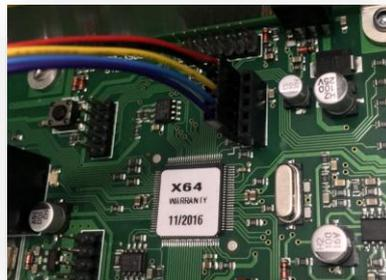
*Tip:* The red wire on the X-Series panel should be closest to the panel's heat sink.
