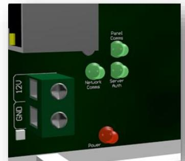
On power up the Network Comms and Server Auth LEDs will flash together, and once it has made a successful connection to the HYYP platform the Server Auth LED will stay on and the Network Comms LED will flash when it's communicating on the network.
